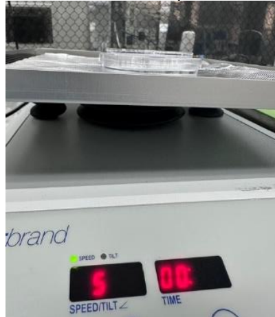
Figure 2. Petri dish with the pillar plates placed on a low-speed rocker.
