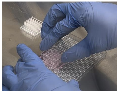
Figure 5. Stamping of the 36PillarPlate on the LoadingPlate to load cells suspended in Matrigel on pillars.
