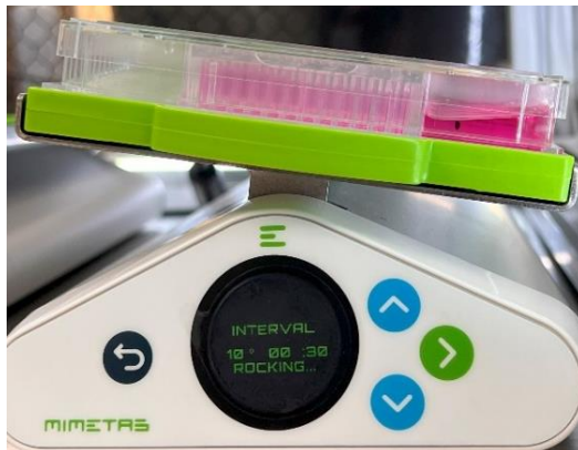
Figure 5. Dynamic cell culture on the 144PillarPlate with the 144PerfusionPlate on the digital rocker at 10° tilting angle with a 30-second tilting angle frequency.
