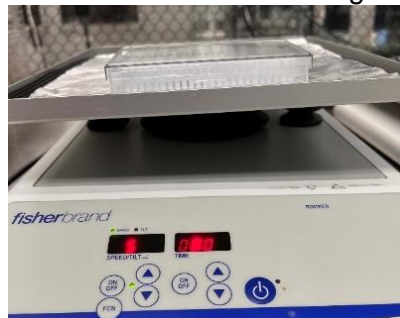
Figure 3. The 384DeepWellPlate with primary antibody on the low-speed rocker at 4°C.
