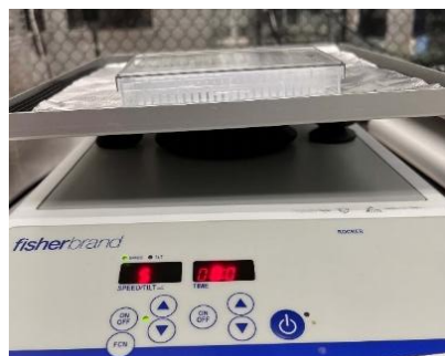
Fig. 11 The 36PillarPlate inserted onto the 384DeepWellPlate with primary antibodies on the low-speed rocker at 4°C for primary antibody staining.
