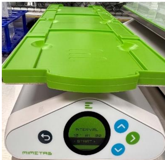
Figure 1. OrganoFlow L digital rocker for loading multiple perfusion plates.
