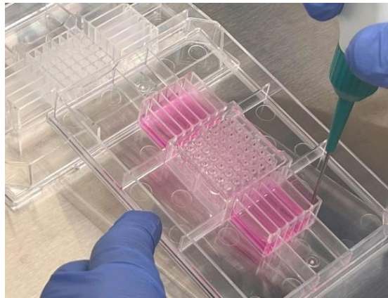
Figure 6. Vacuum aspiration of the old medium from the far end of the lower reservoirs.
