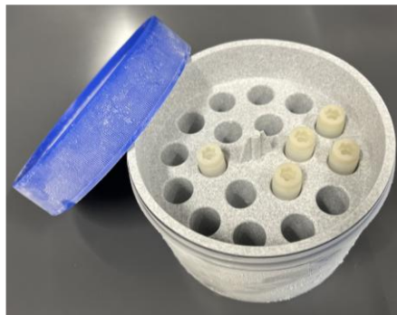
Fig. 4 Freezing cryovials containing iPSCs in the Mr. Frosty container in a - 80°C freezer.
