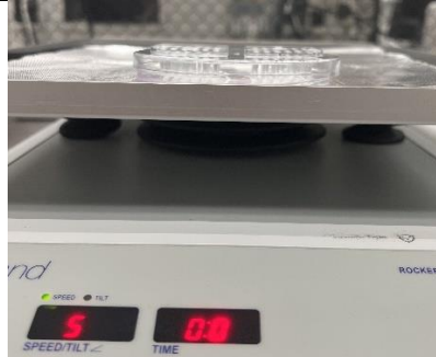
Figure 2. Petri dish with the pillar plates placed on a low-speed rocker.
