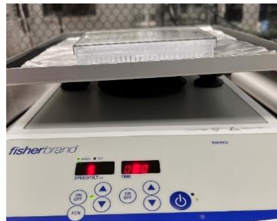
Fig. 11 The 36PillarPlate inserted onto the 384DeepWellPlate with primary antibodies on the low-speed rocker at 4°C for primary antibody staining.
