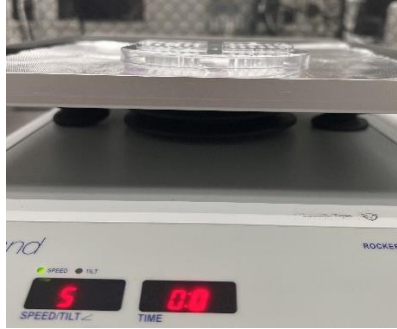
Fig. 10 The petri dish with the pillar plates on a low-speed rocker for permeabilization.
