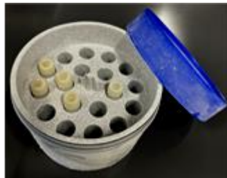
Fig. 3 Freezing cryovials containing iPSCs in the Mr. Frosty container in a - 80°C freezer.
