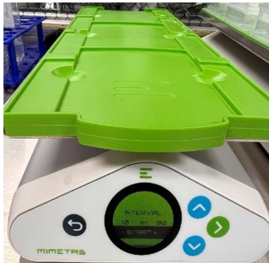
Figure 1. OrganoFlow L digital rocker for loading multiple perfusion plates.
