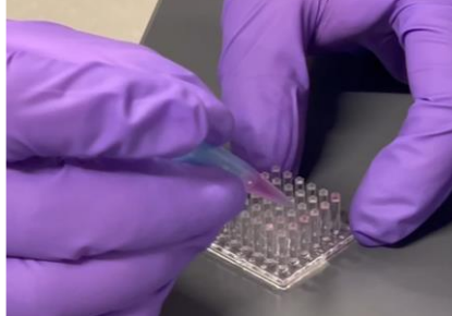
Figure 2. Loading Matrigel on the pillar plate using a 1 mL pipette tip with Matrigel.
