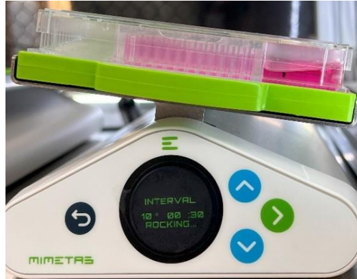
Figure 5. Dynamic cell culture on the 144PillarPlate with the 144PerfusionPlate on the digital rocker at a 10° tilting angle with a 30-second interval.
