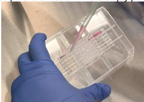
Figure 1. Manual dispensing of a cell growth medium in reservoirs of the 36PerfusionPlate.
