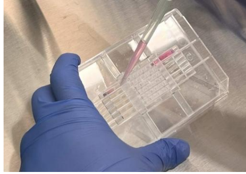
Figure 2. Manual dispensing of a cell growth medium in reservoirs of the 36PerfusionPlate.
