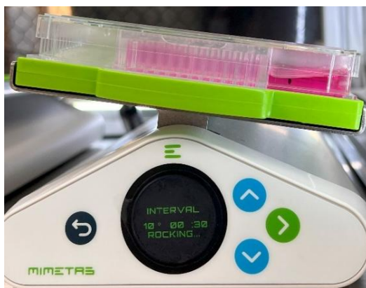
Figure 5. Dynamic cell culture on the 144PillarPlate with the 144PerfusionPlate on the digital rocker at a 10° tilt angle with a 30-second interval.
