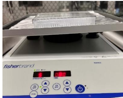
Figure 11. The 36PillarPlate inserted onto the 384DeepWellPlate with primary antibodies on the low-speed rocker at 4°C for primary antibody staining.
