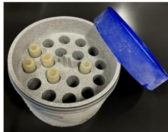
Figure 3. Freezing cryovials containing iPSCs in the Mr. Frosty container in a -80°C freezer.
