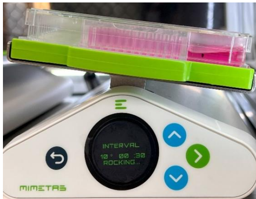
Figure 5. Dynamic cell culture on the 144PillarPlate with the 144PerfusionPlate on the digital rocker at a 10° tilt angle with a 30-second rocking interval.
