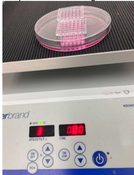
Figure 2. Dynamic cell culture on the 36PillarPlate in a petri dish by rocking the cell culture medium on a low-speed rocker.
