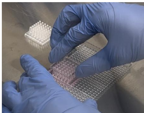
Figure 5. Stamping of the 36PillarPlate onto the LoadingPlate to load cells suspended in Matrigel-alginate on pillars.
